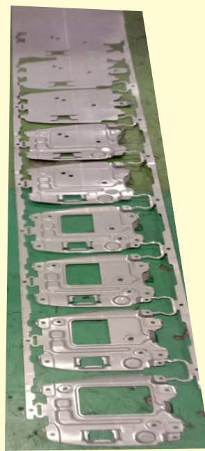
Reinforcement For Car Fuel Lid With Progressive Tools 28000 Pcs / 8 Hrs For Honda Car
