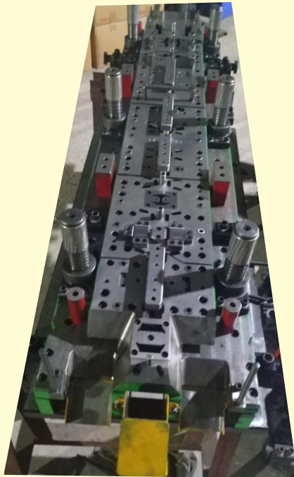
Progressive Tools For Car parts 56000 Pcs / 8 Hrs
