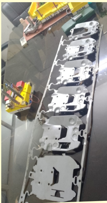
Reinforcement For Car Fuel Lid With Progressive Tools 28000 Pcs / 8 Hrs For Suzuki Car
